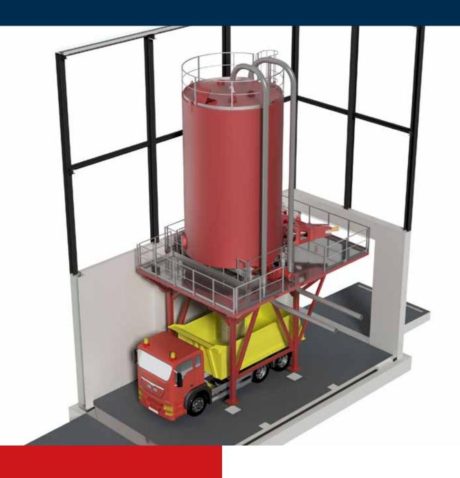
Storage & discharge of centrifuged sludge
